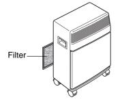
Use a vacuum cleaner to remove the dust on the filter. If the filter is very dirty, dip it in warm water (of less than 40° C.) and rinse it several times. After having washed the filter, let it dry completely before putting it back in place.
